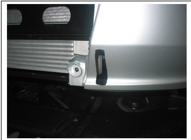
Figure 7 – Completed mounting hole
