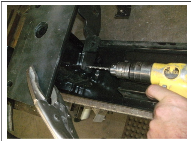
Figure 7 – Drill holes inside of crash can assembly.
