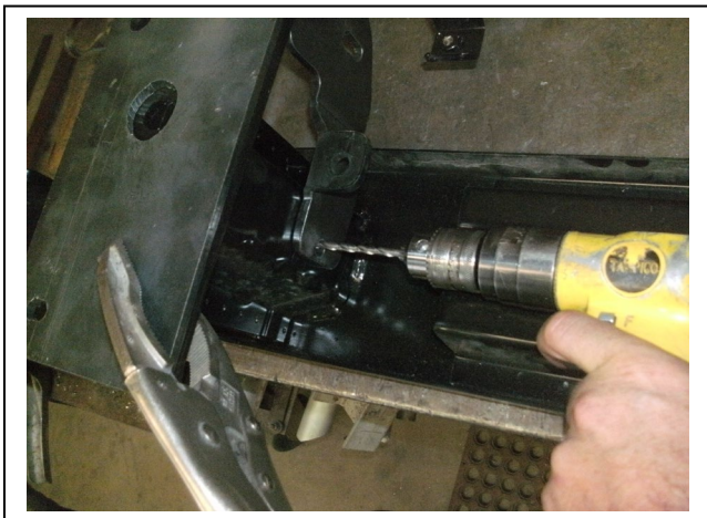
Figure 9 – Drill holes in side of crash can assembly.
