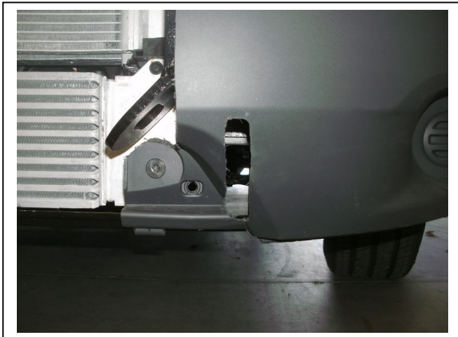
Figure 5 – Completed mounting hole
